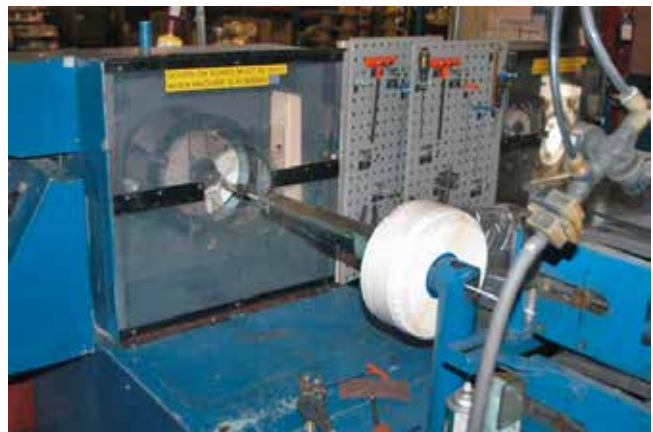
Figure 3. Nomex ® tape being wrapped on the coil conductor.
