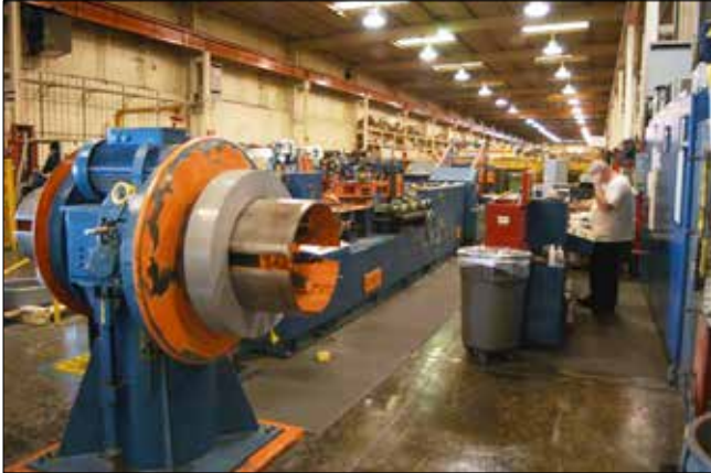
Figure 10. Large Georg core cutter
