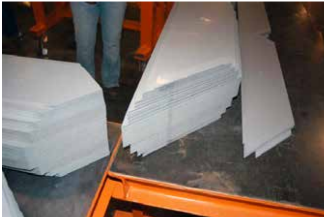
Figure 11. Ends of the middle and outer legs of a step lap mitre cut core.
