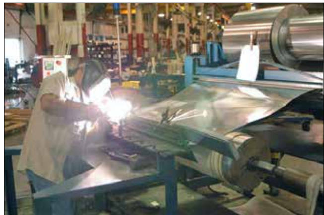
Figure 4. TIG welding LV coil to LV lead.
