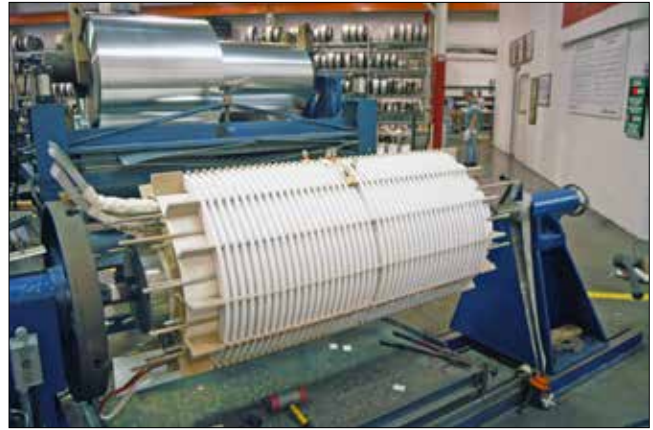
Figure 2. Continuous pancake disk round coil.
