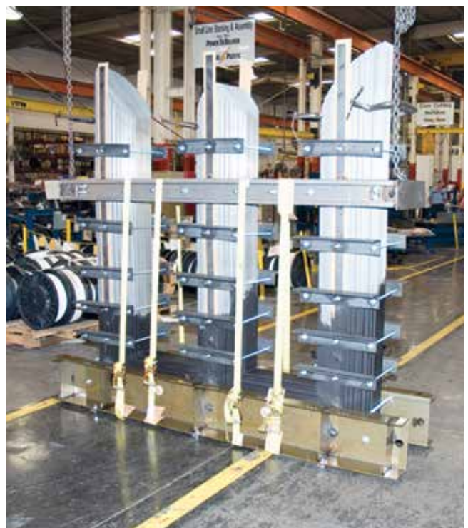
Figure 15. Step-lap mitre core ready for coils.
