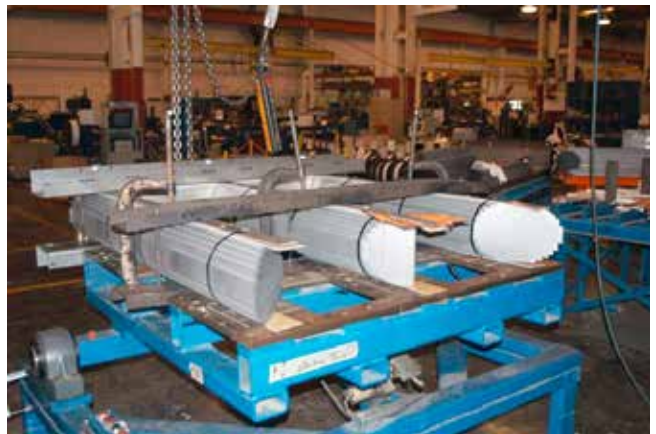
Figure 14. completely stacked core on rotatable table.
