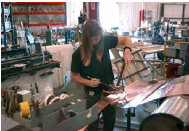
Figure 6. Copper brazing LV coil to LV lead.
