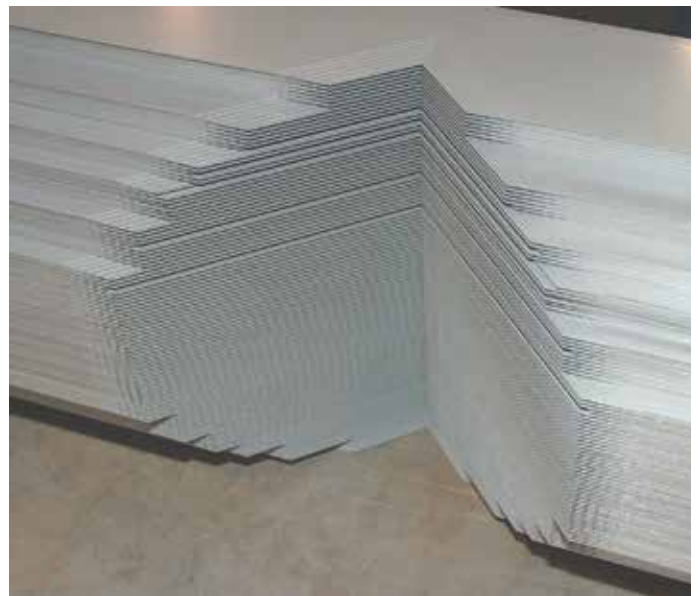
Step-Lap Miter Core Construction
