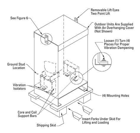
Figure 4 - Typical Assembly for NEMA 1 Enclosures
