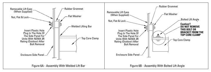
Figure 6 - Shipping Hardware Removal
