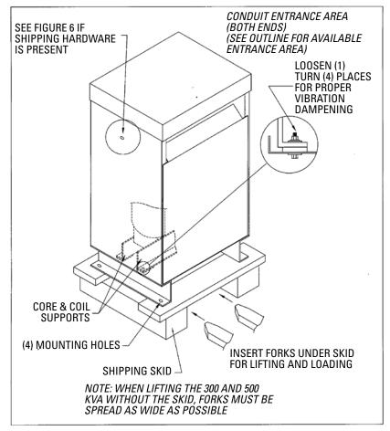
Figure 5 - Typical Assembly for NEMA 2 Enclosures
