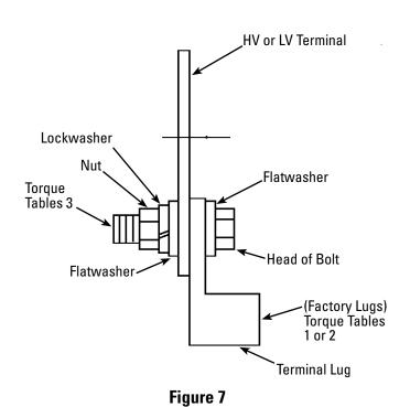
The torque values shown below are for factory supplied lugs only. Use manufacturer requirements for customer supplied lugs. In the absence of manufacturer requirements, refer to torque tables contained in informative Annex I of NEC 2011 or newer. Note — use column B for field installation (column A refers to current cycle testing only).
