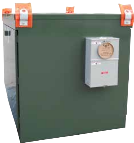
Figure 12. An externally mounted box (see photo at left) for the meter socket with a test switch on the interior is provided on this unit and was specified by this customer. The one-line diagram at right shows that the unit is configured with line and load bushing wells differentiated and arranged for application in a loop scheme (in and out on the line side) and to serve two independent load circuits.
