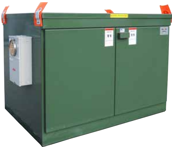
Figure 11. Federal Pacific Primary-Metering Dead-Front unit can be provided with a variety of optional features to accommodate meter sockets, test switches and metering transformers. Labels are provided on the exterior to identify the metering transformer side from the elbow side.
