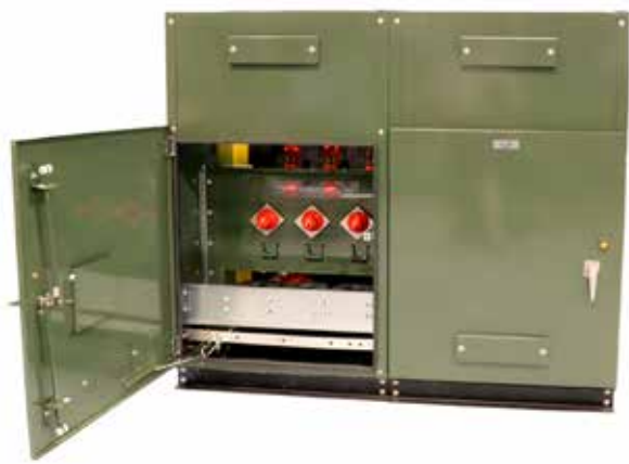
Figure 8. The incoming bushings are shown in photo A at left and the compartment also includes (1) the vacuum fault interrupter that provides switching and protection for the load circuit, (2) the single PT that is connected to Phase B of the incoming circuit and provides control power for the low-voltage components in the control compartment, and (3) the current transformers that provide current sensing for the power monitoring and overcurrent-protection relays. The outgoing bushings are shown in photo B at right and the compartment also includes the three (3) voltage transformers that provide voltage sensing inputs to the power-monitoring relay, which is the revenue metering scheme.
