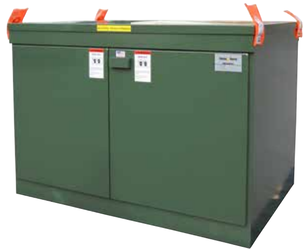
Figure 11. Federal Pacific Primary-Metering Dead-Front unit can be provided with a variety of optional features to accommodate meter sockets, test switches and metering transformers. Labels are provided on the exterior to identify the metering transformer side from the elbow side.
