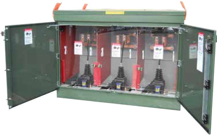
Figure 14. Federal Pacific purchased, installed and wired the outdoor style metering transformers furnished with this unit. In some cases, only mounting provisions are provided for customer furnished and installed metering transformers or, alternately, Federal Pacific will install and wire customer-furnished metering transformers.
