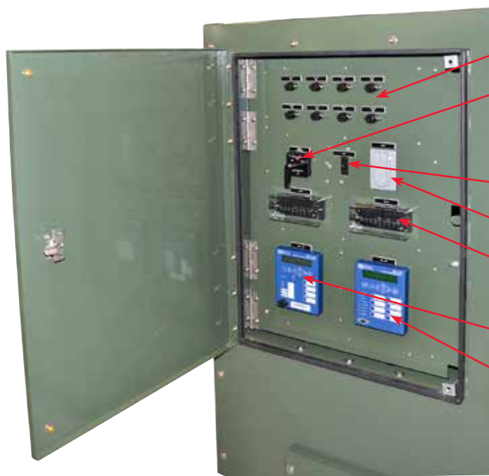
Figure 10. Low-voltage control compartment is mounted integral within the switchgear assembly, but has a separate door and is fully isolated from high voltage. Thus, all operations can be performed without requiring access to the interior of the high-voltage compartment. All controls are surface mounted on a hinged panel making all components and associated wiring readily accessible.
