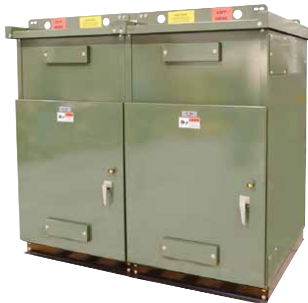
Figure 7. The low-profile, minimum footprint, switchgear assembly pictured above features a vacuum fault interrupter for both load switching and fault interrupting, allowing rapid disconnect of the renewable-energy source from the electric-power utility distribution system whether there is a fault condition on the utility side or the supplier side of grid inter-tie.
