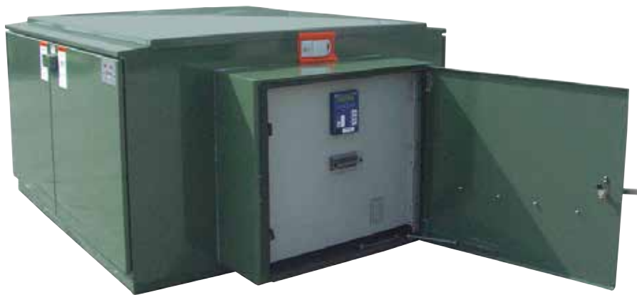
Figure 4. The external low-voltage control compartment is mounted on the side of the unit and includes all of the low-voltage components. The compartment includes a door handle that is padlockable and a wind brace to hold the door open. The door opening is fully gasketed on all four sides to seal the compartment against the weather and contamination. The bottom of the enclosure includes screened vents to allow the interior to breathe with modest air circulation.
