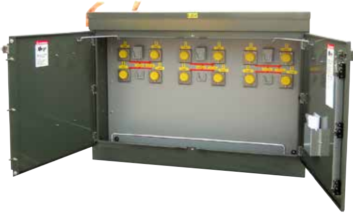
Figure 13. Pictured at left is the dead-front elbow side of the unit. The arrangement shown is phase isolated and the Line and Load bushing wells for each phase are grouped together with Phase A at left, Phase B at center and Phase C at the right. There is suitable label identification for each line-side connection by phase and each load-side connection by phase as well as labels for mimic bus and to identify locations for metering transformers with CTs in series with the bus and VTs tapped from the bus.
