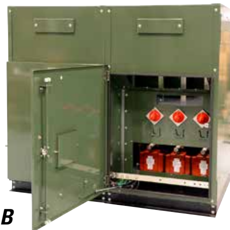
Figure 8. The incoming bushings are shown in photo A at left and the compartment also includes (1) the vacuum fault interrupter that provides switching and protection for the load circuit, (2) the single PT that is connected to Phase B of the incoming circuit and provides control power for the low-voltage components in the control compartment, and (3) the current transformers that provide current sensing for the power monitoring and overcurrent-protection relays. The outgoing bushings are shown in photo B at right and the compartment also includes the three (3) voltage transformers that provide voltage sensing inputs to the power-monitoring relay, which is the revenue metering scheme.
