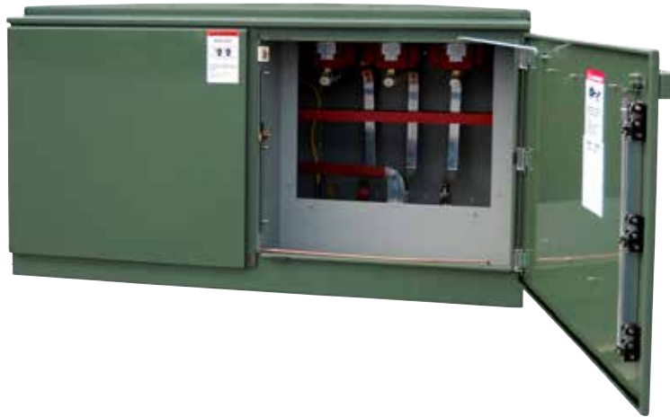
Figure 3. Photo at top shows an open door view of the compartments in which the fused-voltage transformers are mounted. Bolted, removable covers with handle grips allow access to the voltage transformers. The open door view directly above has the access cover removed to allow view of the three-phase set of voltage transformers that provide voltage sensing for the metering function. The single voltage transformer, which is not visible, is mounted in the compartment at the left and is also behind a bolted, removable cover with handle grips. This single VT provides control power to the power-monitoring relay and all the other low-voltage components.
