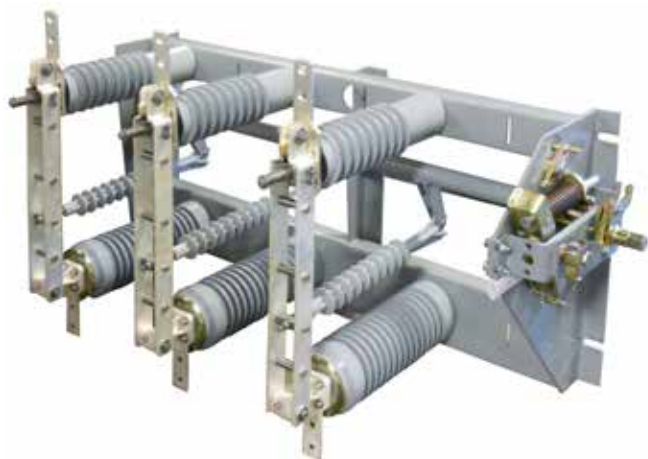
Figure 3. Federal Pacific's 600 ampere 38kV Auto-jet ® Load-Interrupter Switch remains the switching work-horse in the dead-front configuration as it is in all other voltage-class units. The steel operating arm insures fixtured alignment of switch blades and interrupters. Simultaneity of operation of the three interrupters is verified by 100% high-speed videography of the interrupter's performance. Similarly, 100% x-ray of the interrupters and insulators confirm the dielectric integrity of all bushings, bushing wells and insulators.
