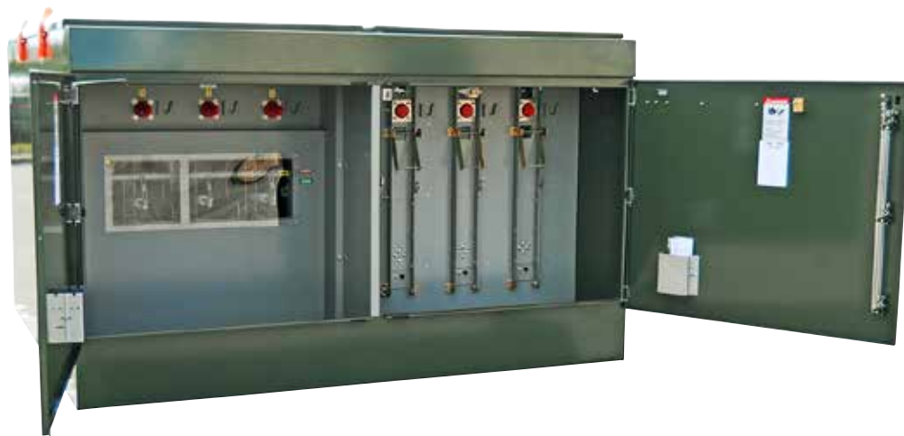
Figure 2. Federal Pacific's 38kV dead-front pad-mounted switchgear is configured virtually the same as the 15kV and 25kV dead-front designs. The switch-termination compartment at left includes 600-amp bushings (at red dust caps) with phase labels, compartment label and adjacent parking stands. A large polycarbonate viewing window allows verification of switch blade position, which is further supported by a switch-position indicator label at the right side of the window – a black arrow (with yellow background) aligns with the open and closed labels to provide visual indication within the termination compartment of the actual switch position. Of course, switch position is absolutely verified by observing the switchblade position through the viewing window. The depth of the switch-termination compartment is adequate to accommodate piggybacked elbows or an elbow with a 200-amp interface to accept elbow surge arresters or grounding elbows.
