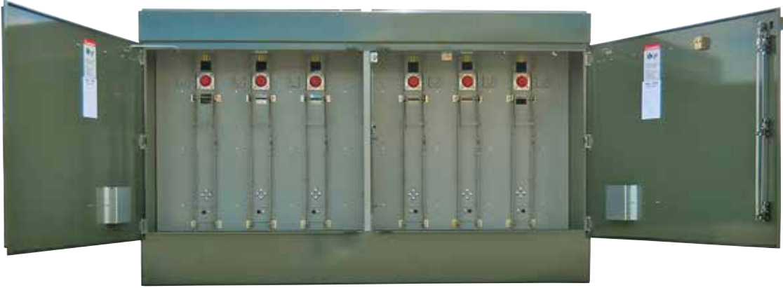
Figure 5. Two of the fuse compartments of the 38kV PSE-12 are pictured above. The fuses are accessed in the same manner as the fuses in all Federal Pacific dead-front units – move the elbow to break the load, raise the latch and pull the fuse panel to pivot down 90° to the horizontal position, lock the fuse panel in place, move the gravity latch away from the contact rod, and push on the end fitting to unlatch the fuse assembly.
