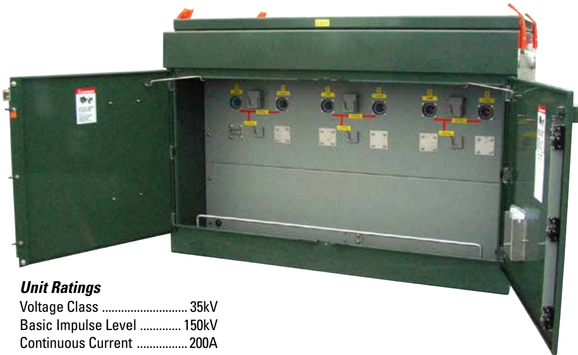
Figure 5. Elbow termination compartment provides 35kV bushing wells to accommodate 200-amp load-break inserts and elbow connectors providing an effective electrical and environmentally secure method to connect power cables to the Primary Metering unit. This unit is furnished as a radial application with one line-side bushing well and one load-side bushing well for each phase. The same unit can accommodate a loop feed arrangement with two line side bushing wells while metering two combined, but independent, load-side circuits as there are (as shown in the above photo) provisions for four bushing wells per phase.
