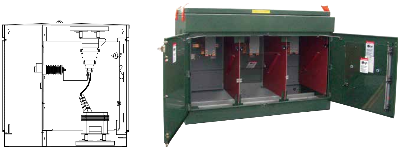
Figure 4. Interphase and end barriers include slides allowing the dual-purpose barriers to be installed in the slide-in position to provide some isolation and separation between CTs and PTs when, for example, changing PT fuses. For units equipped with the automatic door latch, dual-purpose barriers can be stored temporarily behind the latch bar to avoid placing them on the roof or on the ground which may place contamination on the barriers. This unit is also furnished with copper bus and, since the unit is furnished with provisions only for the metering transformers, a painted steel plate is mounted to support the bus during shipment. Adjacent drawing shows a section view from the side of the orientation for the CTs and PTs that the customer expects to install.
