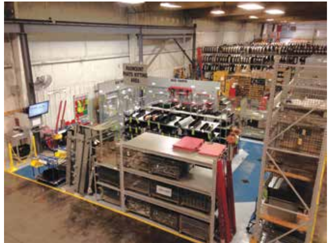
Figure 14 After – Kitting area, using Kanban stocking system.
