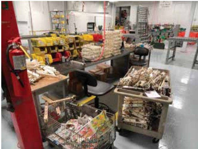
Figure 7 Before – Push production in blade assembly area, resulting in an excess of and potential damage to, in-process material.
