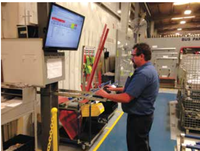
Figure 15 After – Area manager updates the system to display serial numbers of completed parts kit carts, which appear on the monitor.
