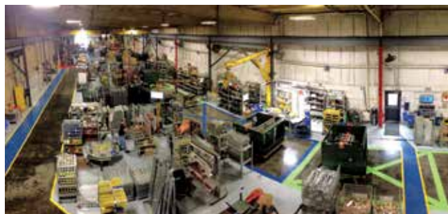
Figure 4 After – The work-station positions (stages) in the pad-mounted switchgear assembly line are clearly marked, with provisions to remove units from the line, if necessary, to avoid production bottlenecks.
