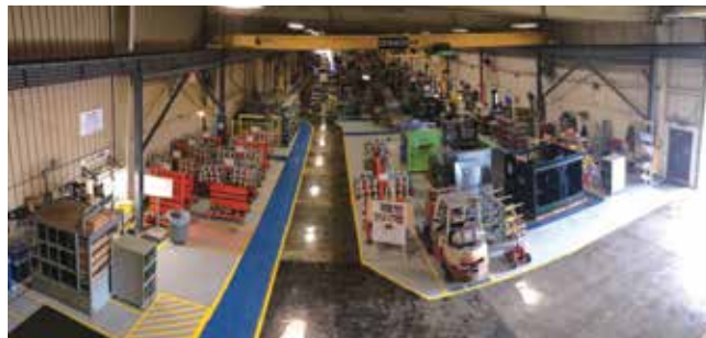
Figure 2 After – The forklift aisle relocation is complete. Only slow-moving inventory remains on the left (background) with sub-assemblies now adjacent to the assembly line. Walkways are marked in blue and lined as separate from the forklift aisle.
