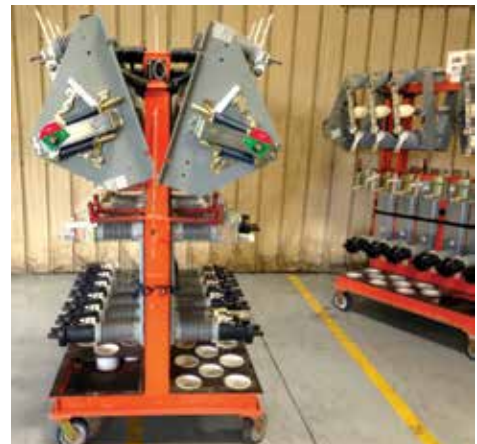
Figure 12 After – Switches and fuse components are produced as needed and are associated with a specific, serially numbered enclosure, by customer job order
