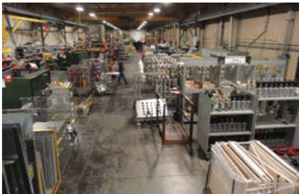
Figure 1 Before – The crowded main forklift aisle accommodated both vehicular and personnel traffic. Active material was stored, and subassemblies were built, at left, across the aisle from the assembly line (at right of picture).
