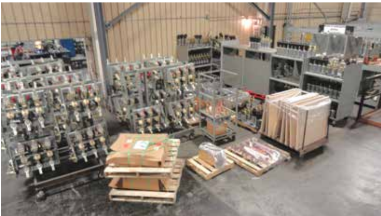
Figure 11 Before – The switches, fuse assemblies and contacts were produced in batches and stored accordingly
