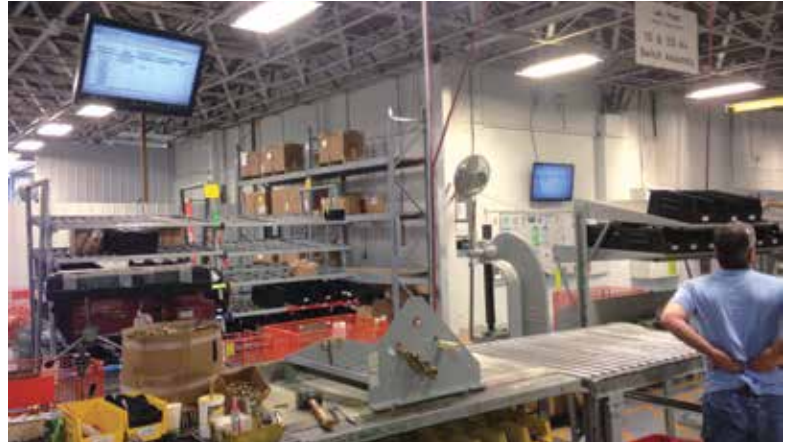
Figure 10 – Monitors in the switch assembly shop show the enclosures being completed. This provides the "schedule" for producing switch and fuse component assemblies that are to be installed in those specific enclosures.
