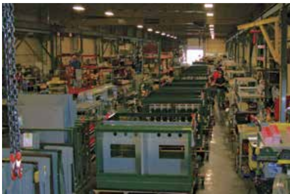
Figure 3 Before – A view of the pad-mounted switchgear assembly line (to the right of the forklift aisle) is unmarked and without apparent order.
