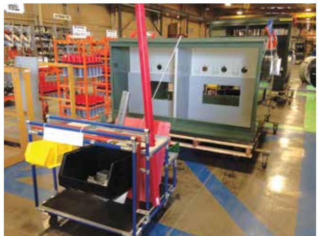
Figure 16 After – Parts kit cart is matched to its associated enclosure on the assembly line.
