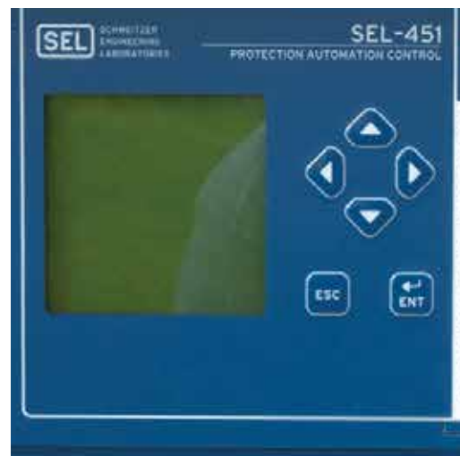
Figure 9. The LCD screen presents the continuously scrolling primary display points. In addition, soft keys facilitate navigation among the primary display points and the “Main Menu Screen”, which provides additional display points for the “EVENTS”, editing of the “DATE/TIME” and initiating the “DISPLAY TEST” to illuminate all LEDs to confirm that the lamps are functional.
