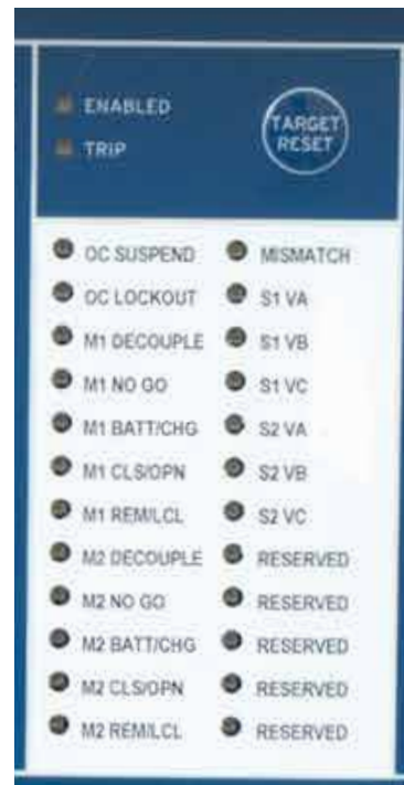
Figure 10. Twenty-four Status LEDs are provided to give actual status of key functions. The various LEDs and the associated functions are illustrated above. In addition, the "ENABLED" LED provides indication that the SEL-451 relay is powered on and the "TRIP" LED illuminates when the relay has initiated a transfer operation
