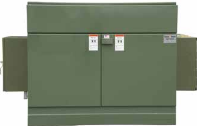
Figure 1 – Exterior view of a typical four-compartment Federal Pacific ATPSE-9-44222 15kV Automatic Source-Transfer Pad-Mounted Dead-Front Switchgear. The “9” configuration, as shown in this illustration, configured with two three-phase source switches and two three-phase sets of load fuses, is the most common configuration for Pad-Mounted Automatic Source-Transfer Switchgear.
