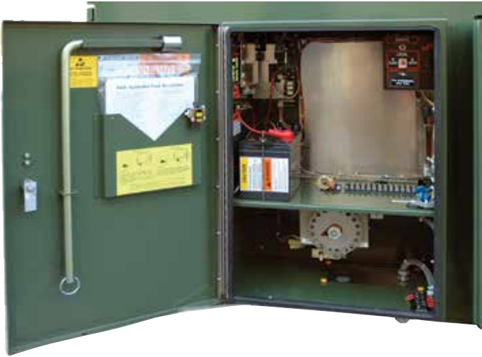
Figure 4. The Federal Pacific Run-and-Trip motor operator, as illustrated above, provides automation for Federal Pacific Auto-jet® II load-interrupter switches. Federal Pacific motor operators have the reliability essential to providing power to critical loads. These motor operators include a decoupler to allow testing without affecting service continuity to the load; and a long-life battery and battery charger to insure functionality even when the control-power source is not available, which are just a few of the many important features furnished.
