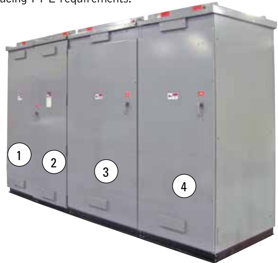
Figure 1. This six-bay lineup of 25kV Manual Metal-Enclosed Switchgear is arranged in a back-to-back configuration with four (4) bays in the front (in the two top photos taken from the left side and from the right side) and two (2) bus-transition bays in the rear (in the photo at left). The configuration allows the medium-voltage distribution switchgear with a vacuum circuit breaker to better match the available space at the installation site.
