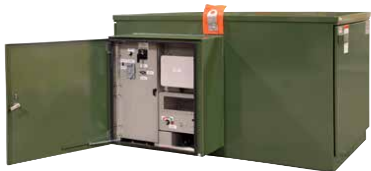
Figure 2. Open door view of the Low-Voltage Control Compartment on the PVE-5 that includes a 15kV MAVRiC® with a Self-Powered Relay to provide switching and protection for a load-feeder circuit. Other relay types, which may require a control-power source for operation, are also available.
