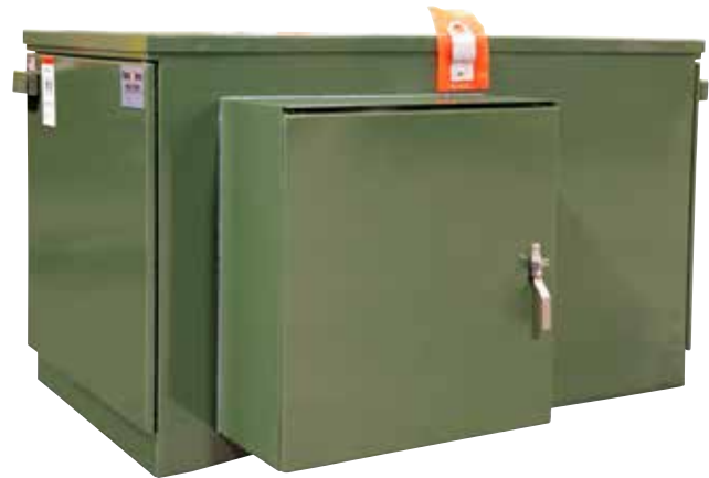
Figure 1. View of PVE-5 that includes a 15kV MAVRiC® — combines a vacuum circuit breaker with an integral In-Line visible disconnect. Low-voltage compartment on side includes, Self-Powered Overcurrent Relay, viewing window to inspect visible disconnect; vacuum circuit-breaker control handle; manual handle for operation of visible disconnect and selector switches and indicators. See Figure 4 for complete details of all items in low-voltage control-compartment. All control functions are isolated from medium voltage, including elbow connectors and cables. There is never a need to enter the cable-termination compartments unless it is necessary to access cables and elbow connectors.
