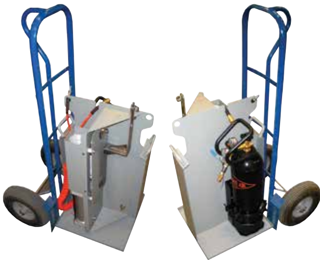
Figure 13. Portable remote operating mechanism available from Federal Pacific can be mounted over handle on switchgear stile and operated from a distance of up to 50 feet to open and close the switch using compressed air or CO 2 . Similar arrangements are available for pad-mounted switchgear.
