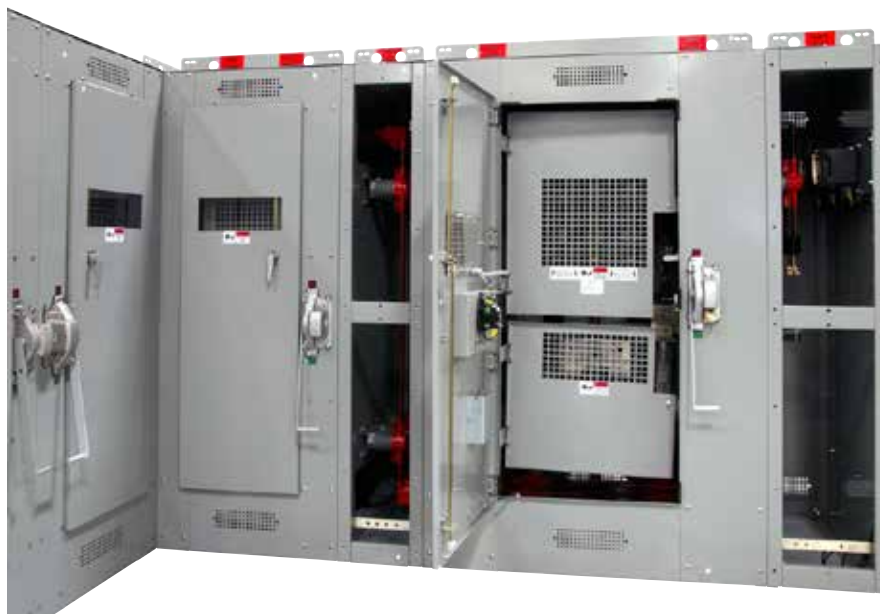
Figure 4. In certain situations, the incoming switch may be open and the circuit is served from the other source, but the fuses in this main compartment still remain energized. Consequently, separate screens are provided over the main switch and over the main fuses. This is done to prevent immediate direct access to the fuses and labels provide a reminder that the fuses may be energized.
