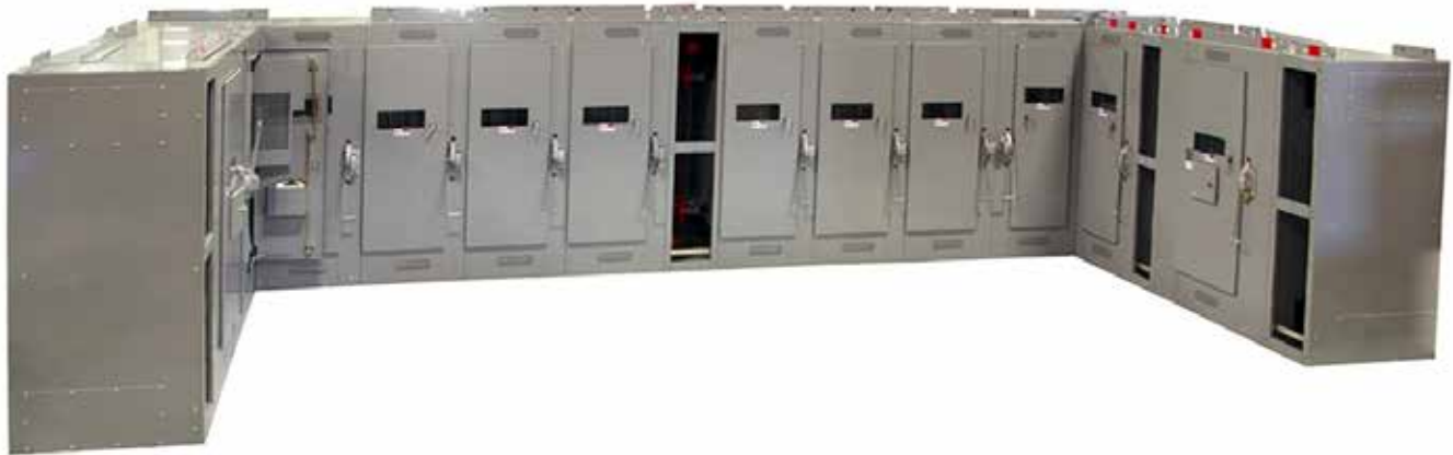
Figure 1. A 19-bay switchgear assembly configured in a U-shaped arrangement is pictured above nearing completion. Open bays, which are incoming-termination compartments on each end and bus-transition sections on interior units, are closed off with cover plates. This indoor assembly matches to available room size at the installation and minimizes expense associated with capturing floor space from rental or production area for utility services at any facility.
