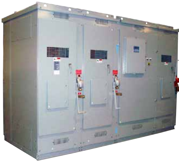
Figure 1. Federal Pacific Metal-Enclosed Switchgear in a four (4) bay configuration features (from left) two incoming switch-only bays for primary-selective service (and also serve as the line side visible disconnect for the vacuum switch), a bay containing a vacuum switch and a switch/fuse feeder bay that provides circuit protection for the load circuit as well as providing a load-side visible disconnect for isolating the vacuum switch when maintenance service is required.
