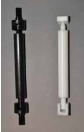
Figure 10. Federal Pacific has developed a new turnbuckle, which is connected between the fuse panel and the red GPO-3 fiberglass shutter barrier. The enhanced design (in black) has increased mechanical capability and is easier to install, remove and replace. It can be used to replace installed earlier-design turnbuckles, requiring only the addition of a suitably-sized hole in the barrier.
