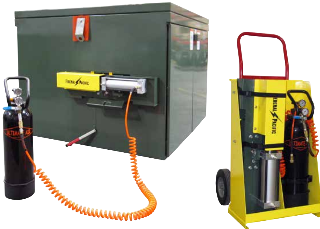
Figure 7. Federal Pacific's Portable Remote Operating Mechanism is transported on a two-wheel cart to the unit. The support bracket is mounted in the existing switch-operating handle pocket without requiring any modification of the enclosure and without requiring any tools. The air cylinder is mounted on the support bracket; the air hose is connected to the air cylinder and the CO 2 tank, which is moved away from the unit and the tank opened with the gas pressure released by turning a valve opening/closing the switch.
