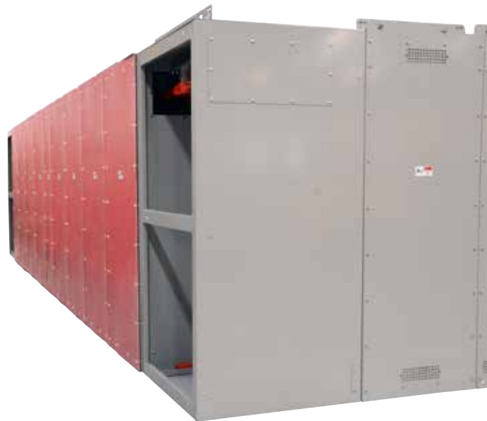
Figure 17. A 19-bay switchgear assembly configured in a U-shaped arrangement is pictured above nearing completion. Open bays, which are incoming-termination compartments on each end and bus-transition sections on interior units, are closed off with cover plates. This indoor assembly matches to available room size at the installation and minimizes expense associated with capturing floor space from rental or production area for utility services at any facility.
