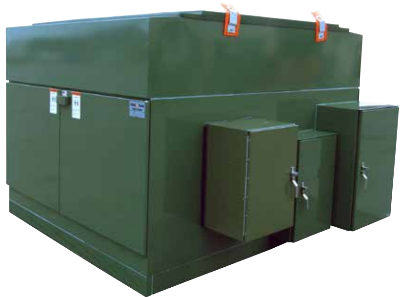
Figure 6. The Dead-Front Automatic-Transfer ATPVE-9 pictured and diagramed above provides primary-selective service to critical loads at the user's installation utilizing Federal Pacific Auto-jet®II Load Interrupter switches. Switching and protection of the load circuits is provided by relayed vacuum circuit breakers with visible disconnects.
