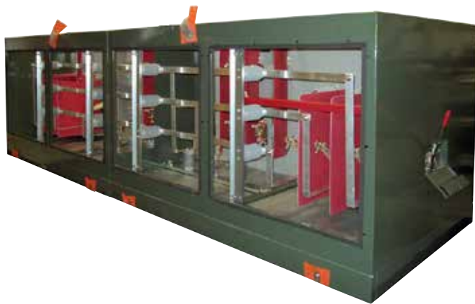
Figure 4. The rear of the unit with the close-off covers removed is pictured above along with a three-line circuit diagram of the single-side PSE-9. Gasket is installed around all four sides of each opening. Tamper-resistant hardware will secure the covers in position and compress the gasket to seal each opening against entry of moisture or contamination. The main interconnecting bus runs along the rear of the unit. The switch-operating handle is shown with the cover removed and the handle in position for operating the switch.
