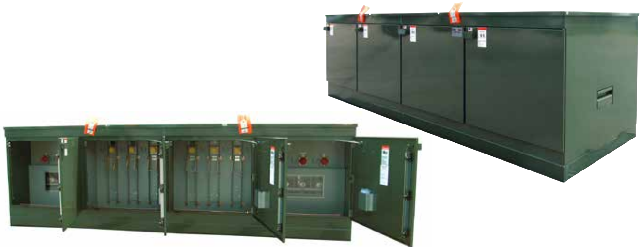
Figure 3. Pictured above are photographs of the single-sided PSI/II-9 unit. This unit will find particular application in locations where a narrow lot line exists, where operating space is limited and where other conditions dictate the advantage of having all cable connections and fuse operation on one side with switch operation not requiring exposure to cables.
