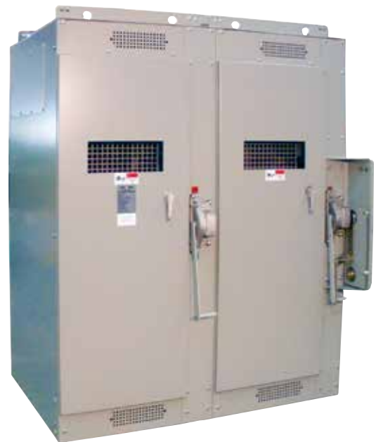
Figure 20. Metal-enclosed switchgear (and pad-mounted Switchgear not pictured) is shown equipped with a Federal Pacific Portable Remote Operating Mechanism on the bay at right to allow operation from a distance of up to 50 feet using compressed air or CO 2 .
