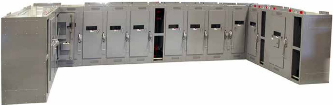
Figure 17. A 19-bay switchgear assembly configured in a U-shaped arrangement is pictured above nearing completion. Open bays, which are incoming-termination compartments on each end and bus-transition sections on interior units, are closed off with cover plates. This indoor assembly matches to available room size at the installation and minimizes expense associated with capturing floor space from rental or production area for utility services at any facility.
