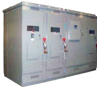
Figure 14. Federal Pacific Metal-Enclosed Switchgear in a four (4) bay configuration features (from left) two incoming switch-only bays for primary-selective service (and also serve as the line-side visible disconnect for the vacuum switch), a bay containing a vacuum switch and a switch/fuse feeder bay that provides circuit protection for the load circuit as well as providing a load-side visible disconnect for isolating the vacuum switch when maintenance service is required. The one-line diagram is below.
