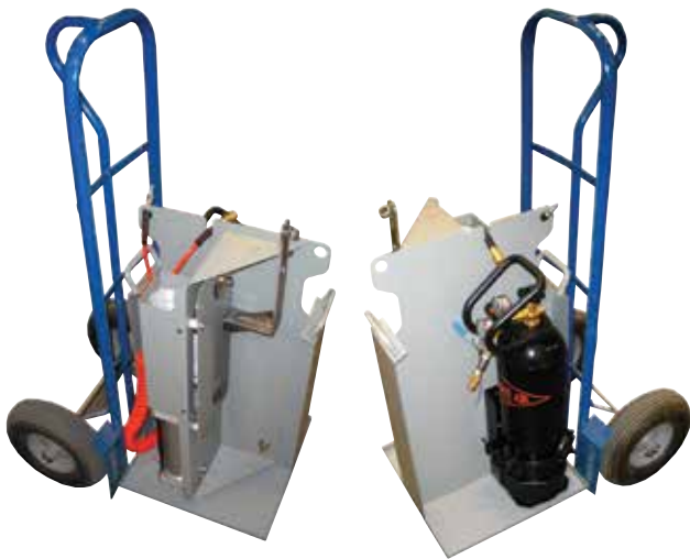
Figure 19. Portable remote operating mechanism available from Federal Pacific can be mounted over switch-operating handle on switchgear stile and operated from a distance of up to 50 feet to open and close the switch using compressed air or CO 2 . Similar arrangements are available for pad-mounted switchgear.
