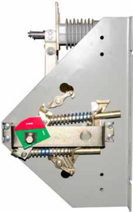
Figure 9. Switch-operating mechanisms of Federal Pacific 15kV Auto-jet®II load-interrupter switches now incorporate stainless-steel springs. These high-performance springs offer significant enhancement over the springs previously used especially in resistance to corrosion as proven in salt-spray testing as well as in mechanical performance as proven by exhaustive mechanical testing, including timing tests. The top photo shows the two springs with the solid blue spring being the old-style spring. The stainless spring has only a partial blue overspray applied for differentiation from other springs in the factory. The stainless steel springs are shown installed on a switch in photo at bottom left and the old style are shown on the switch at bottom right.
