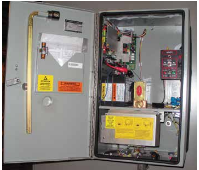
Figure 3. Fast-Trip Style Type PM Motor Operator has a larger, high-speed motor and space to accommodate an array of communications and control components similar to the Standard-Style Motor Operator. Cover (with yellow label) over motor is interlocked so that when the cover is open, motor operation is blocked to prevent exposure to fast moving parts.
