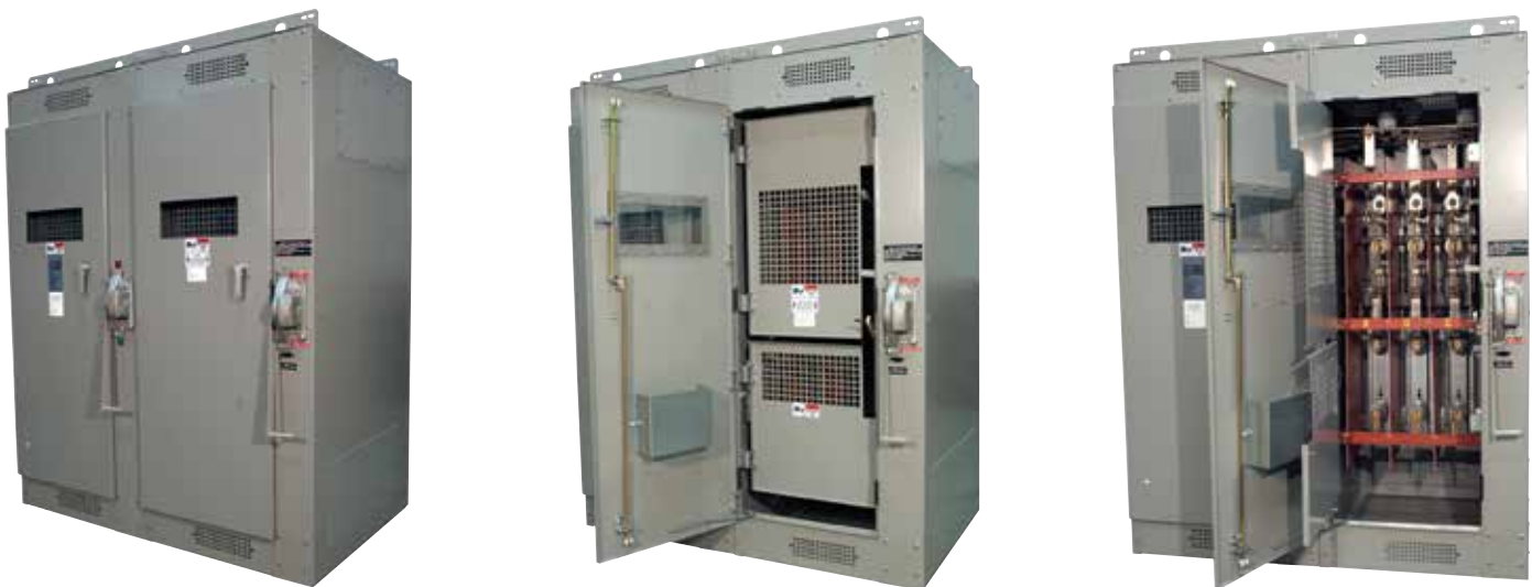
Pictured above are typical feeder bays with automatic-trip (shunt-trip) switches, providing feeder isolation when a single-phase condition (such as a blown feeder fuse) occurs.
