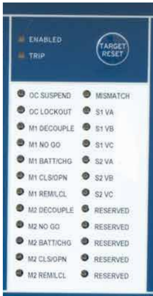
Figure 3. Twenty-four Status LEDs are provided to give actual status of key functions. The various LEDs and the associated functions are illustrated above. In addition, the "ENABLED" LED provides indication that the SEL-451 relay is powered on and the "TRIP" LED illuminates when the relay has initiated a transfer operation.
