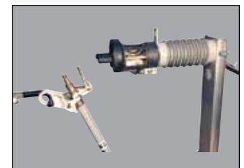
Holder parted, Auto-jet® reset for next operation.
