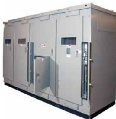
Figure 1. Type ME Motor Operators are mounted in the switchgear stile, adjacent to the compartment door opening and allowing the enclosure width to remain at only 36 inches. Federal Pacific's source-transfer relay is mounted on the switchgear in a separate low-voltage enclosure. As pictured above, the SEL-451 relay is mounted on the compartment door of the second bay from right.
