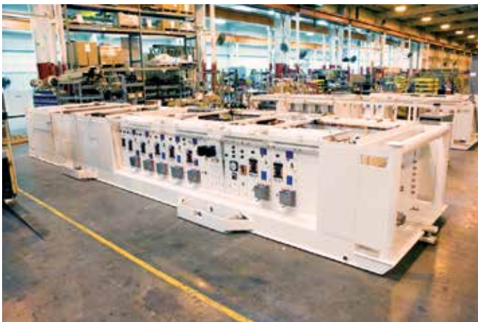
Figure 11. A 1500-kva portable power center nears completion with wheel fittings for railroad wheels or tread tires is shown in the photo above.
