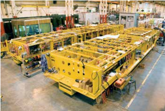
Figure 5. Sophisticated, highly automated totally self-contained power-delivery systems, incorporating the widest range of electric power components, are developed, designed, fabricated, finished, assembled, tested, transported, off-loaded and provided with start-up service engineered and systems checkout.
