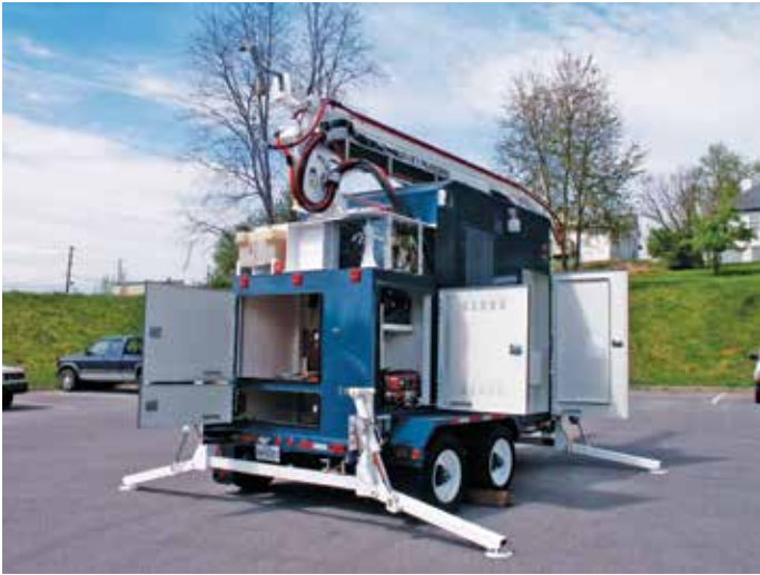
Figure 15 Towable portable substation includes all control and hydraulic articulated boom with cross-arm — shown with boom extended in Figure 16.
