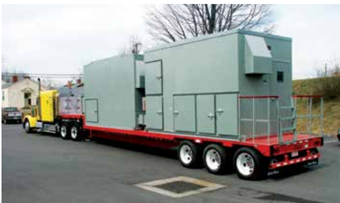
Figure 13. Totally enclosed heavily insulated substation is destined to provide alternate power source while servicing installed substation on Alaskan oil pipeline systems.
