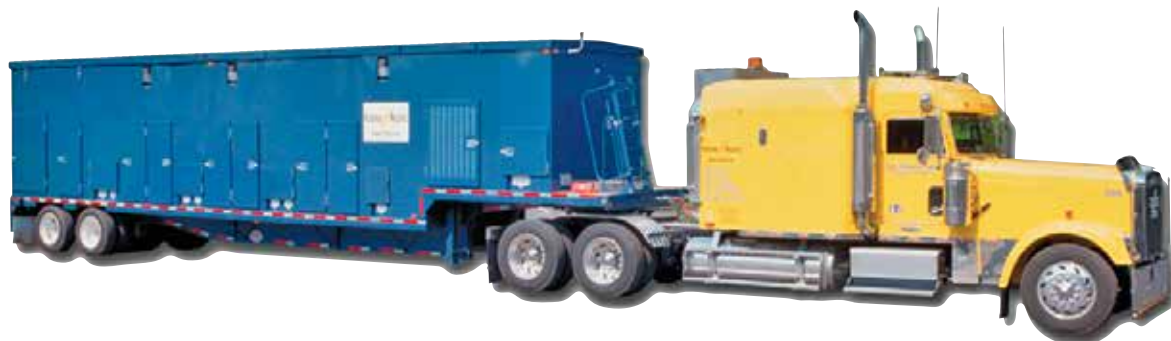
Figure 18. Trailer-mounted, totally enclosed distribution substation matched to emulate an installed base of vaults allows vaults to be by-passed for repairs or replacing components without loss of power to the customer during a planned intervention or in an emergency break.
