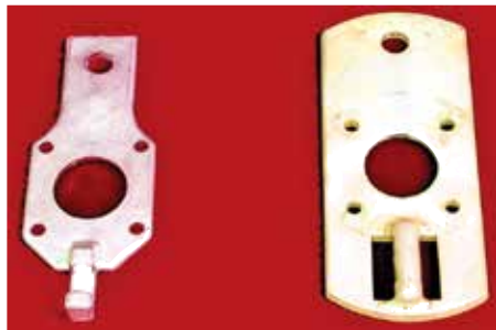
Figure 4. For loadbreak fuse mountings, view shows present cast fuse main contact at left and previous main contact, which was a weldment, at right (removed from fuse mounting).
