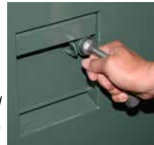
Figure 4. Door handle cover is secured closed by a penta-head (or hex-head) bolt. Turn socket counter-clockwise to loosen bolt. Do not use power tools.
