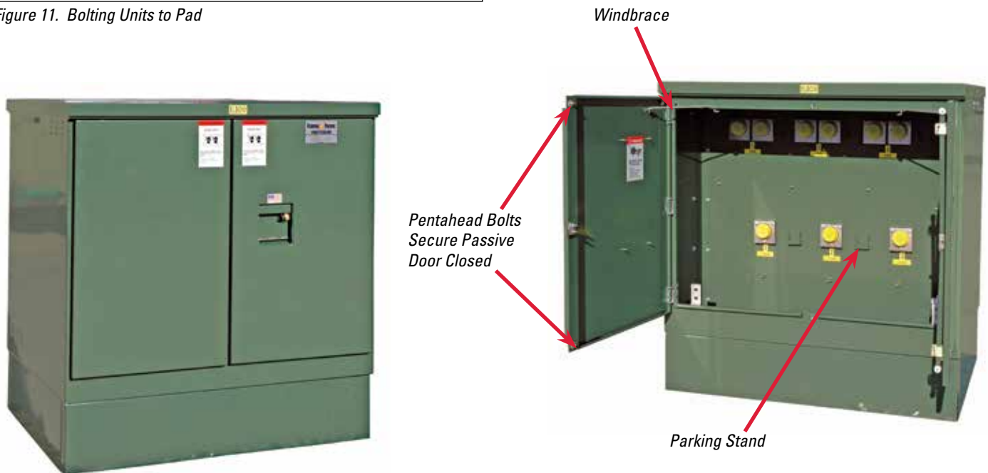
Figure 12. Views of FTDF elbow-compartment side with doors closed (at left) and open (at right) to show customer selected bushing wells (pictured) or, if specified optional 600-ampere bushings. The 200-ampere bushing wells accommodate loadbreak inserts and elbow connectors. Dust covers (yellow discs) must be removed from all unused positions and replaced with protective insulating bushing-well plugs (or bushing covers when furnished with 600-ampere bushings, which have red dust covers).
