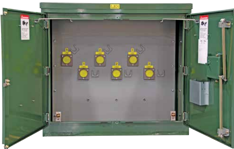
Figure 6. View of PMDF elbow-compartment side with doors open to show customer selected bushing wells (pictured) or, if specified optional 600 ampere bushings. The 200 ampere bushing wells accommodate load-break inserts and elbow connectors. Dust covers (yellow discs) must be removed from all unused positions and replaced with protective insulating bushing-well plugs (or insulating bushing covers when furnished with 600 ampere bushings, which have red dust covers).
