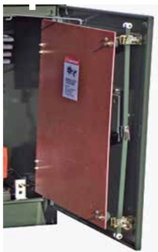
Figure 12. Three-point door latch mechanism. Enclosure door is secured open by windbrace. Inner barrier is secured open by a pin on the door inserted into a clip on the barrier.
