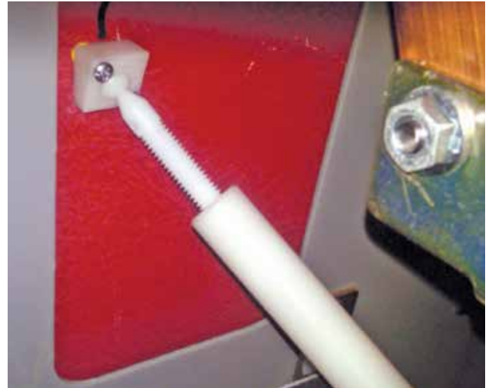
Figure 6. Turn the barrel of the Sliding Rod Assembly and thread it approximately halfway on the Ball Rod.
