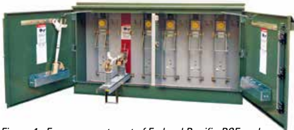
Figure 1. Fuse compartment of Federal Pacific PSE pad-mounted switchgear. Spacing between fuse panels is adequate to accommodate a horizontal feed-thru standoff bushing - and there is a viewing window directly in front of each fuse, making blown-fuse targets fully visible. Doors feature three-point automatic, self-latching door latches. The captive security bolt rotates 60° in either direction (clockwise or counter-clockwise) to open. Do not use power tools. See page 4 for additional information
