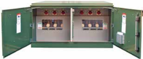
Figure 2. Switch compartment of Federal Pacific PSE pad-mounted switchgear. Storage for fuse assemblies is on fuse side, better facilitating fuse changing procedures. Wide-view windows and broad blades provide improved visibility to make it easier to verify switch position, even behind cables and elbows, while the open/closed labels serve to further enhance this user-friendly design.
