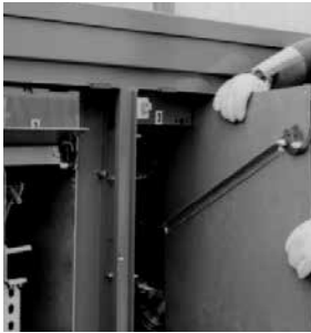
Figure 8. Switch and fuse side removable barriers facilitate cable installation and termination when the switchgear is de-energized. Fuse side is shown. Lift up until rivets on barrier align with slot in top front barrier guide, and pull out to remove barriers.
